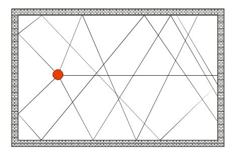
The level decreases exponentially and will be linear in a logarithmic display. The reverberation time is the decay constant.
