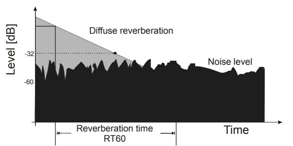
In most cases the decay is measured to a lower value –significantly above the noise level- e.g. -32dB and then extrapolated to -60dB.
