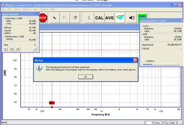
You should now avoid any ambient noise. Once, you pressed OK, Akulap waits for the trigger signal.
