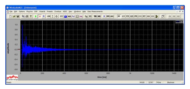
With such linear display, we can monitor this impulse response up to 600ms. Therefore it is more useful to use a logarithmic display, which is called Energy Time Curve (ETC). We can clearly see the linear decay for the diffuse part.
