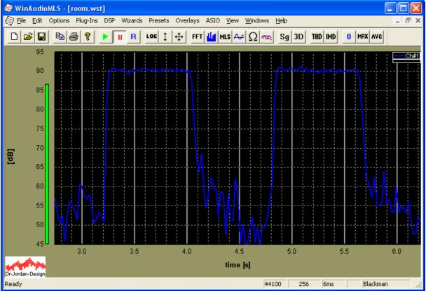
This method is still simple and is implemented by many hand-held devices. Since any other noise has direct impact on the measurement, high sound levels are required. This requires special designed loudspeaker and amplifiers. In addition, this method is only used to measure the reverberation time and not the impulse response.
