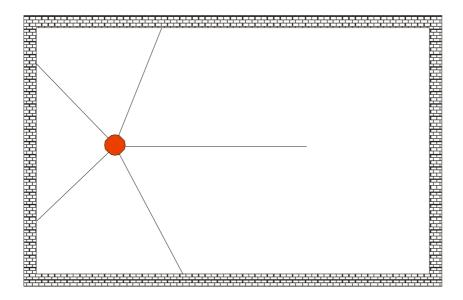
Once it reaches a wall, the wave is reflected changing its level, phase and direction.
