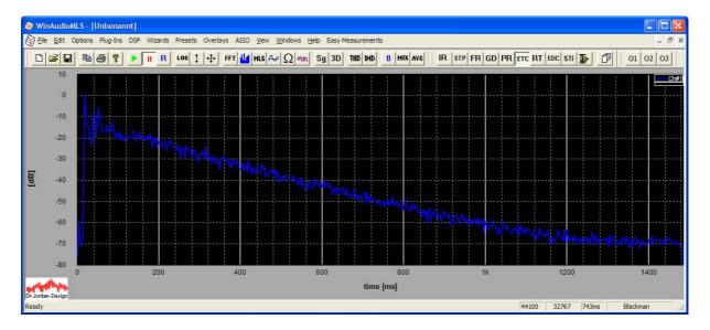
The most important plot is the Schröder plot (Energy Decay Curve, EDC), which is the basis for reverberation calculation. In this example, we selected a range from -5dB to -45dB as a basis for calculation of RT60. For this example, we get a wide-band reverberation time RT60 of 1.3s.
