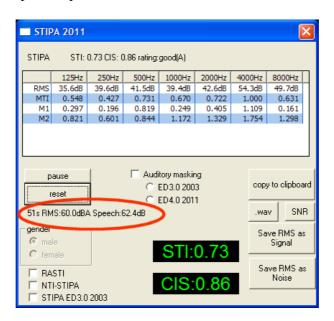
In this window you get the normal A-weighted RMS reading, which is basically the energy-equivalent average over the measurement time (here 51s).
