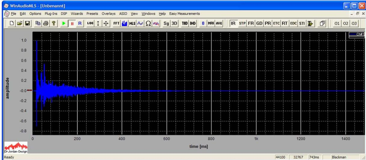
With such linear display, we can monitor this impulse response up to 600ms. Therefore it is more useful to use a logarithmic display, which is called Energy Time Curve (ETC). We can clearly see the linear decay for the diffuse part.
