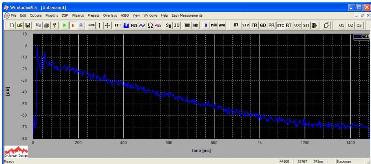
The most important plot is the Schröder plot (Energy Decay Curve, EDC), which is the basis for reverberation calculation. In this example, we selected a range from  $-5\text{dB}$  to  $-45\text{dB}$  as a basis for calculation of  $\text{RT}_{60}$ . For this example, we get a wide-band reverberation time  $\text{RT}_{60}$  of 1.3s.
