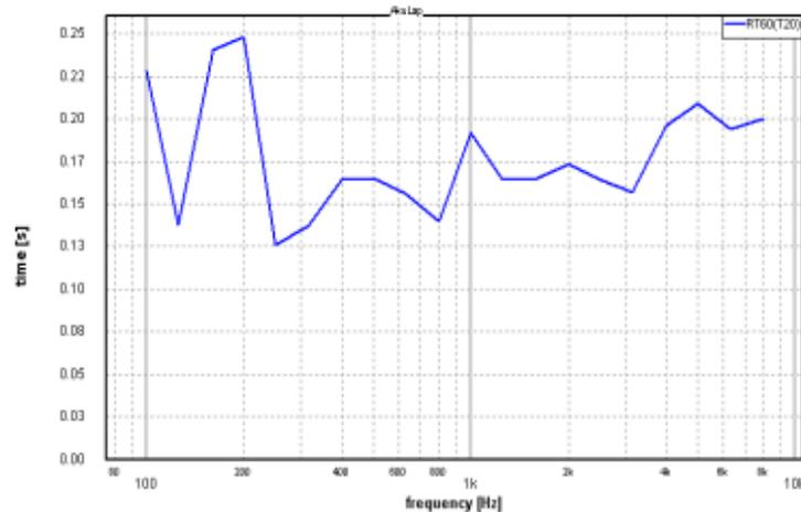
reverberation time wide-band 83Hz to 9600Hz: RT60(T20)=0.16s
