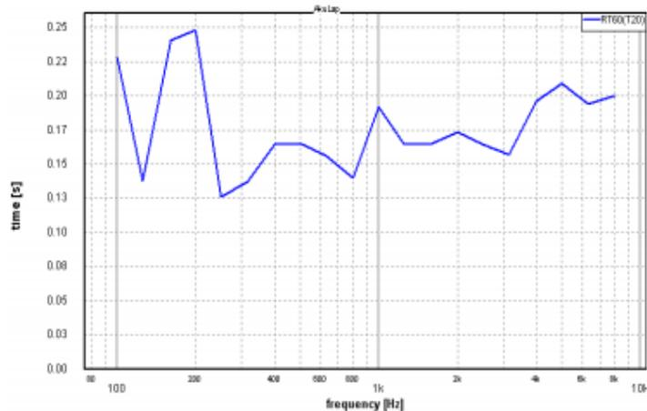
reverberation time wide-band 83Hz to 9600Hz: RT60(T20)=0.16s
