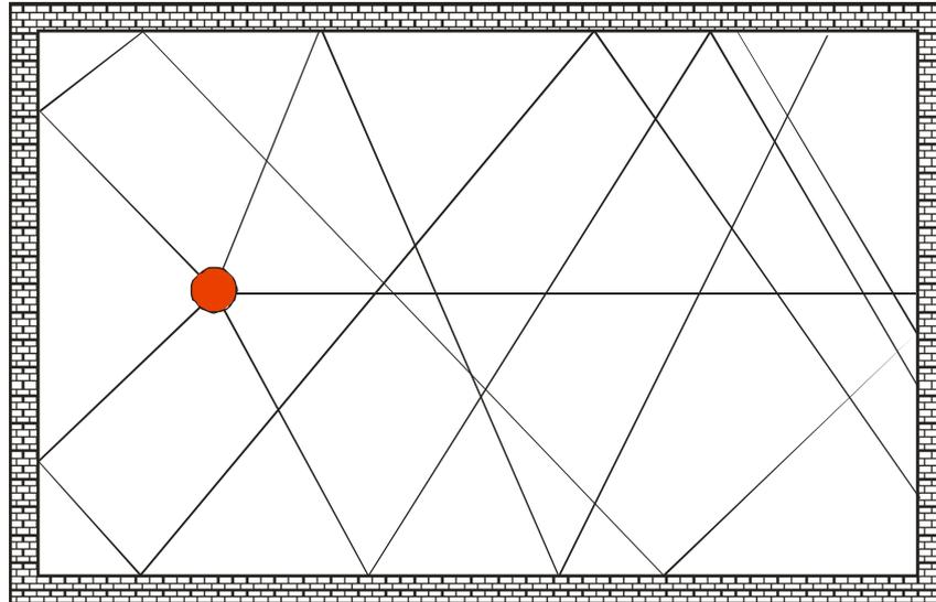
The level decreases exponentially and will be linear in a logarithmic display. The reverberation time is the decay constant.
